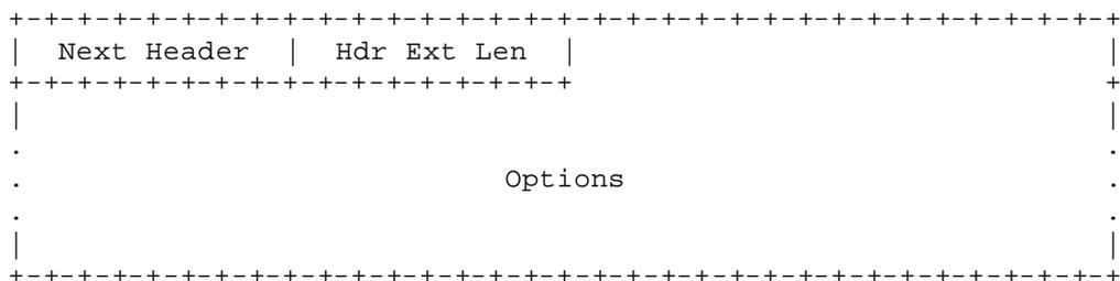
The first three bits of the first byte are zero and the value 5 in the remaining five bits is the Hop-by-Hop Option Type number. By zeroing all three, this specification requires that, nodes not recognizing this option type should skip over this option and continue processing the header and that the option must not change en route.
