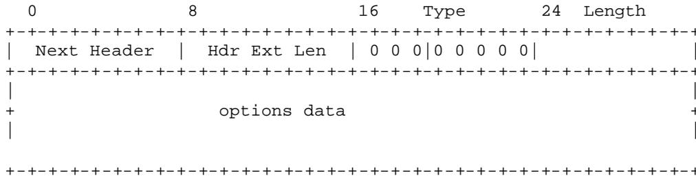
There are a total of 8 possible combinations out of which the IntServ model uses two. The rest can be can be exploited by the DiffServ model and future use.
