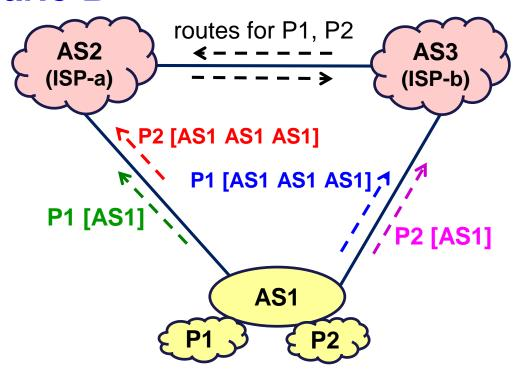
Consider data packets received at AS2 with source address in P1 or P2:
