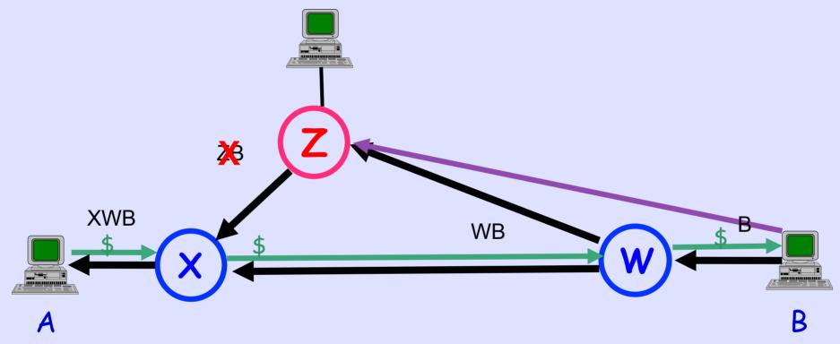
B cryptographically signs the message to W Sb(B->W)
