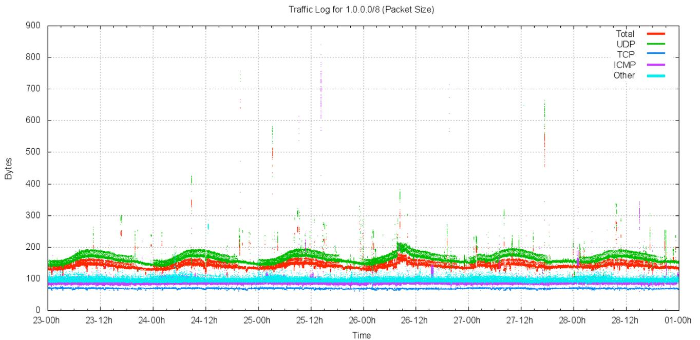
Figure 8 – Distribution of Packet Sizes by Protocol
