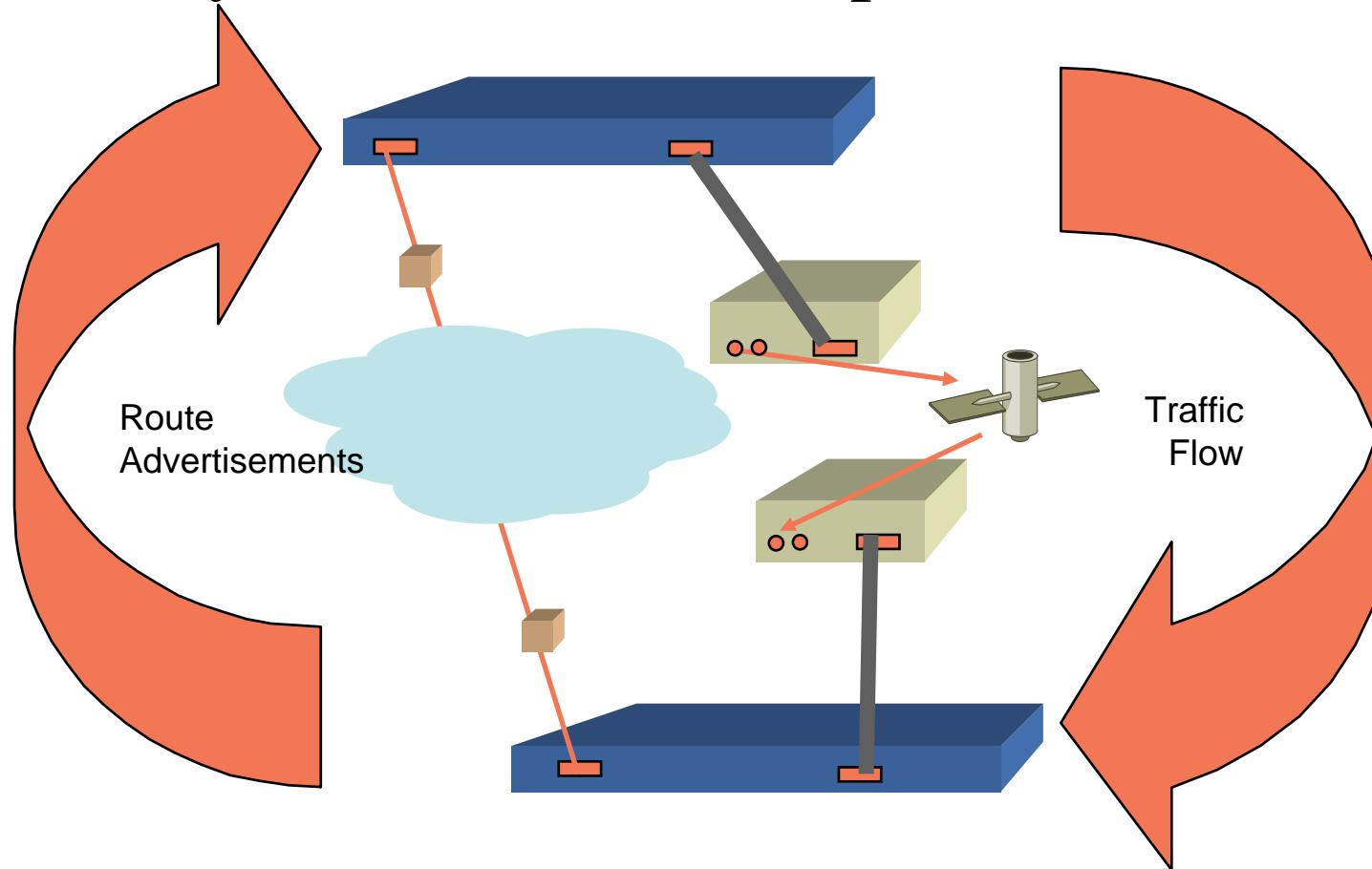
Any break in the unidirectional circuit will cause a BGP keepalive failure, which in turn will cause the BGP session to fail. This eliminates the need for an HDLC keepalive signal along the satellite path
