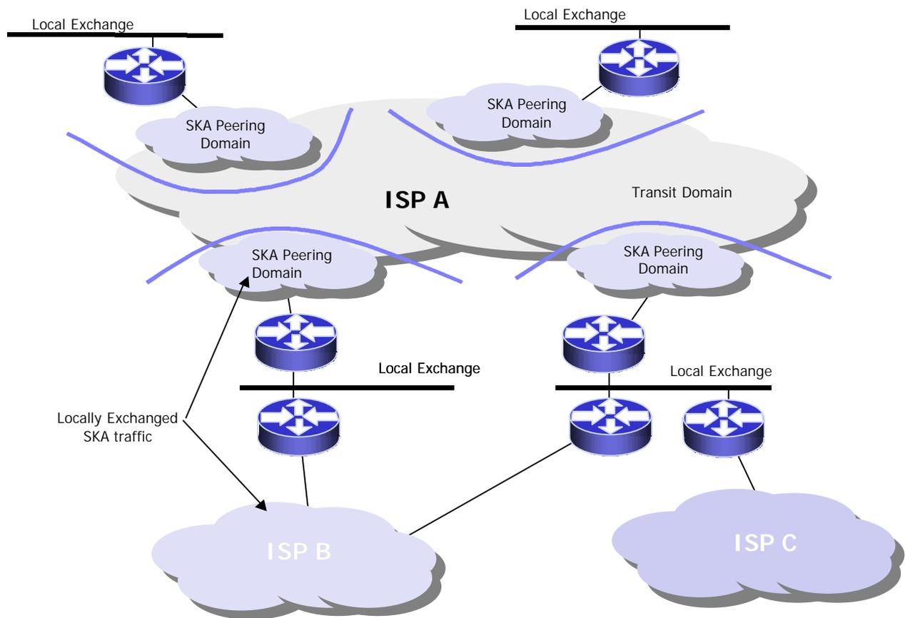
**Figure 12. SKA peering using local cells.**
