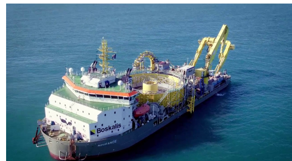
Figure 6 – A Cable Laying Ship
