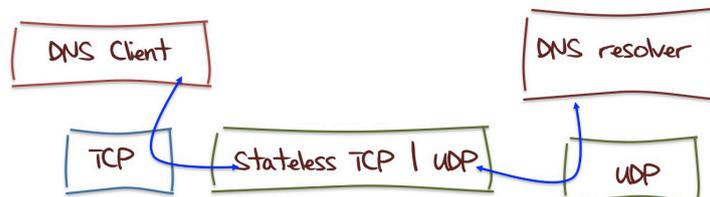
The stateless TCP / UDP DNS proxy server pick up clients' DNS queries in TCP and directs them via UDP to a DNS resolver, and provides the response again using TCP.
