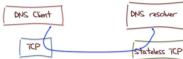
This has much the same properties of the hybrid model, and just could be coerced into working. But then again I'm not keen to start hacking around inside an implementation of a DNS server, so the fastest way to prototype this approach is to put in a TCP / UDP translator between the client and the server:
