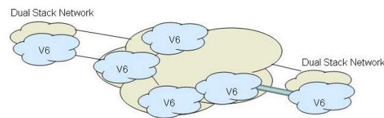
It might be the case that at some stage there would be a phase when network infrastructure may be IPv6 only, in which case there would also be some use of tunnelling IPv4 over IPv6 to ensure continuation of ubiquitous connectivity.
