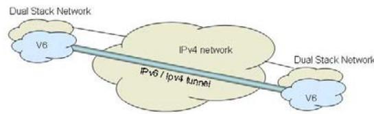
Progressive stages of the transition would see these IPv6 "islands" interconnect directly, and also see the commencement of the older IPv4-only networks converting to a dual stack environment.
