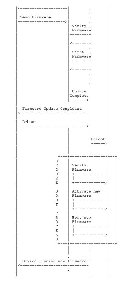
Figure 2: First Example Flow for a Firmware Update
