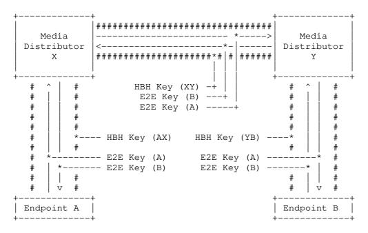
Figure 2: E2E and HBH Keys Used for Authenticated Encryption of SRTP Packets
