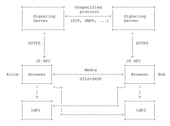
Figure 4: A Federated Call with IdP-Based Identity
