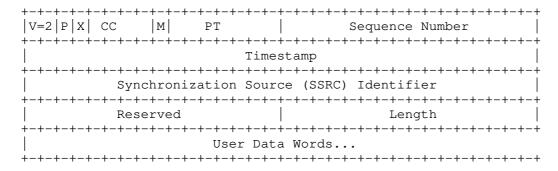
Figure 1: RTP Payload Format for TTML
