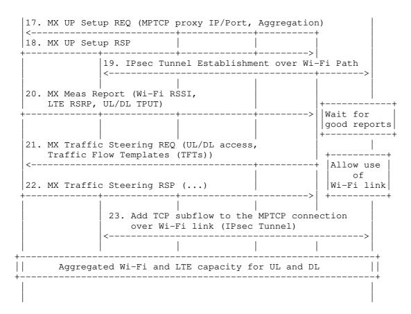
Figure 19: MAMS-Assisted MPTCP Proxy as User Plane - Add Wi-Fi Leg
