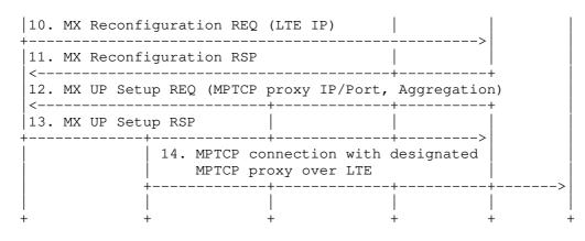
Figure 18: MAMS-Assisted MPTCP Proxy as User Plane - Initial Setup with LTE Leg
