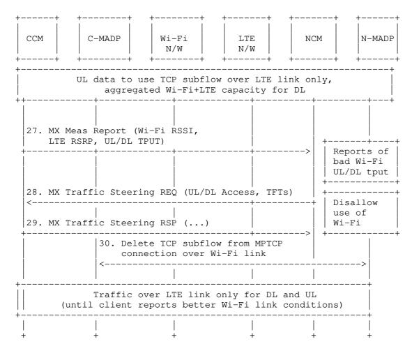
Figure 21: MAMS-Assisted MPTCP Proxy as User Plane - Part 4
