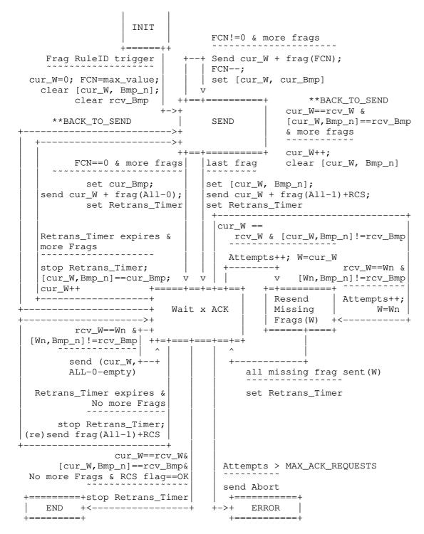
Figure 43: Sender State Machine for the ACK-on-Error Mode
