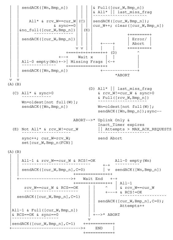
Figure 44: Receiver State Machine for the ACK-on-Error Mode
