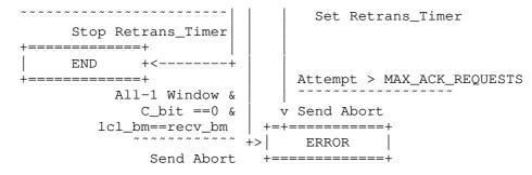
Figure 41: Sender State Machine for the ACK-Always Mode
