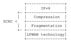
Figure 2: Example of Protocol Stack Comprising IPv6, SCHC, and an
