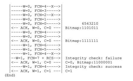
Figure 34: ACK-Always Mode, 11 Tiles, One Tile per SCHC Fragment, Three Lost SCHC Fragments
