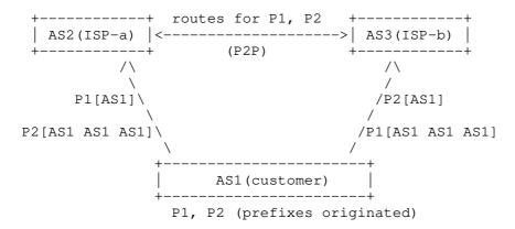
Consider data packets received at AS2 via AS3 that originated from AS1 and have a source address in P1:
