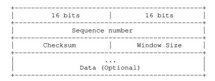
Figure 6: Transport Protocol Data Packet Format
