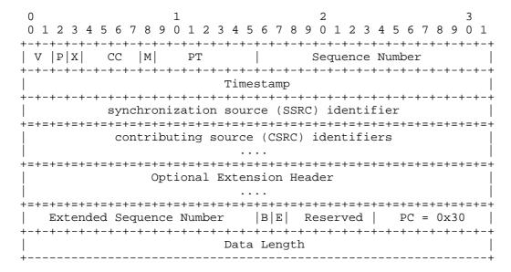
Figure 6: RTP Payload Format for Padding Data
