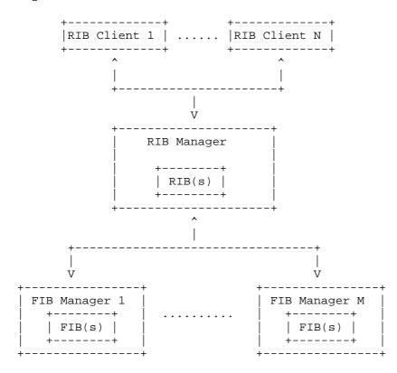
Figure 1: RIB Manager, RIB Clients, and FIB Managers
