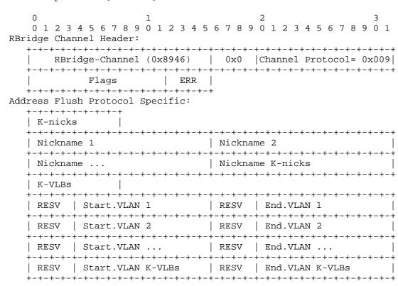
Figure 2: Address Flush Message - VLAN Block Case
