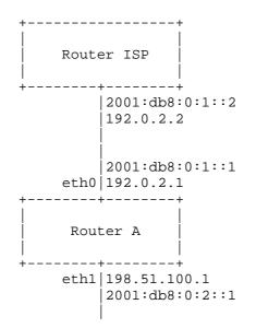
Figure 2: Example of Network Configuration
