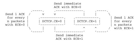
Figure 1: ACK Generation State Machine
