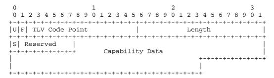
Flag "U" MUST be set to 1 to indicate that this capability must be silently ignored if unknown. The TAC's Capability Data field contains the Targeted Application Element (TAE) information, encoded as follows:
