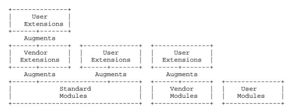
Figure 2: YANG Module Origin Types
