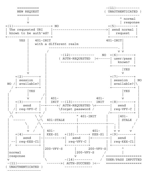
Figure 5: State Diagram for Clients
