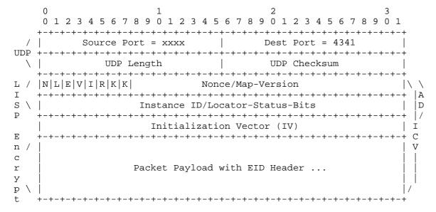
K-bits Indicate When a Packet Is Encrypted and Which Key Is Used
