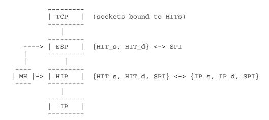
Figure 2: Architecture for HIP Host Mobility and Multihoming
