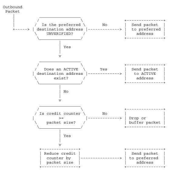
Figure 9: Sending Packets with Credit-Based Authorization
