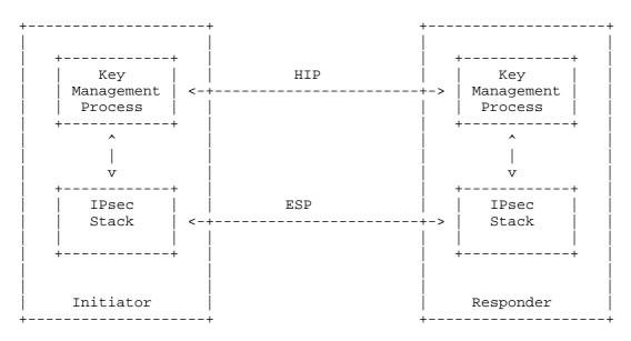
Figure 1: HIP Deployment Model
