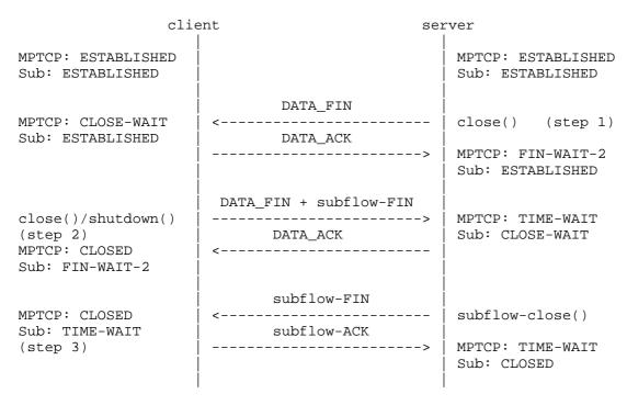
Figure 5: Multipath TCP may not be able to avoid time-wait state on the subflow (indicated as Sub in the drawing), even if enforced by the application on the client-side.
