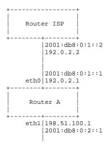
Figure 3: Example of Network Configuration
