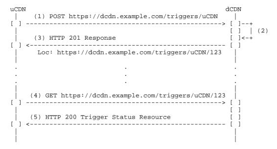
Figure 1: Basic CDNI Message Flow for Triggers
