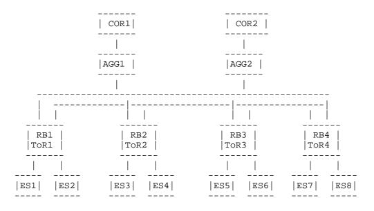
Figure 1: A Typical TRILL DC Network
