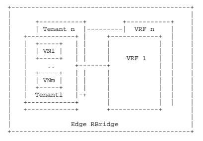
Figure 2: Edge RBridge Model as Distributed Gateway
