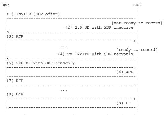
Figure 7: SRS Responding to Offer with a=inactive
