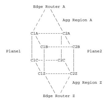
Figure 2: Dual-Plane Network and Disjointness
