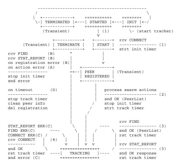
Figure 5: "Per-Peer-ID" State Machine and Flow Diagram
