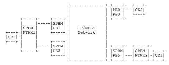
Figure 1: PBB and SPBM EVPN Network
