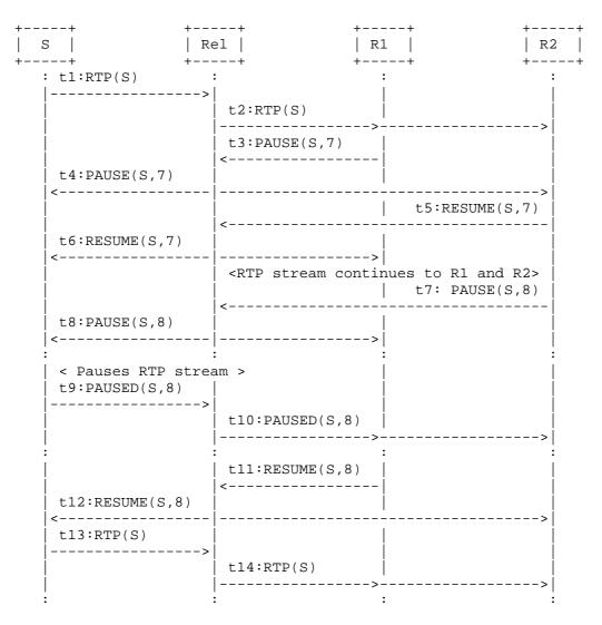
Figure 19: Pause and Resume Operation between One Sender and Two Receivers through Relay
