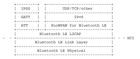
Figure 3: IPv6 and IPSS on the Bluetooth LE Stack
