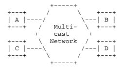
Figure 5: Point to Multipoint Using Multicast
