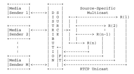
FT = Feedback Target Transport from the Feedback Target to the Distribution Source is via unicast or multicast RTCP if they are not co-located.
