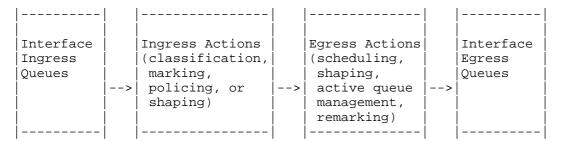
Figure 1: Generic Traffic Management Capabilities of a Network Device
