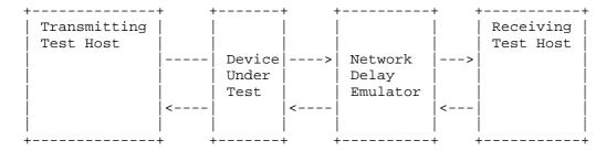
Figure 2: Lab Setup for Traffic Management Tests
