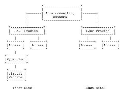
Figure 2: SARP: Network Architecture Example
