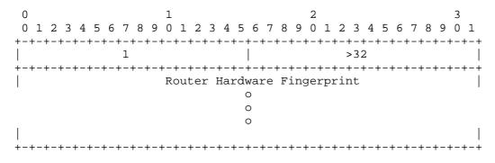
Router-Hardware-Fingerprint TLV Format
