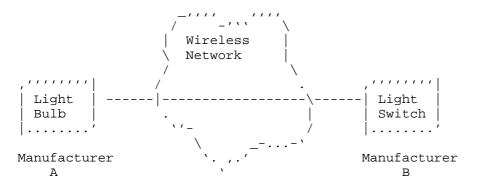
Figure 1: Device-to-Device Communication Pattern
