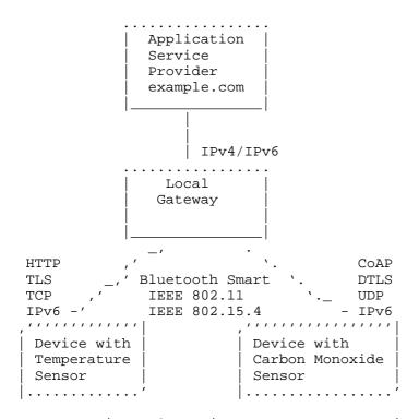
Figure 3: Device-to-Gateway Communication Pattern
