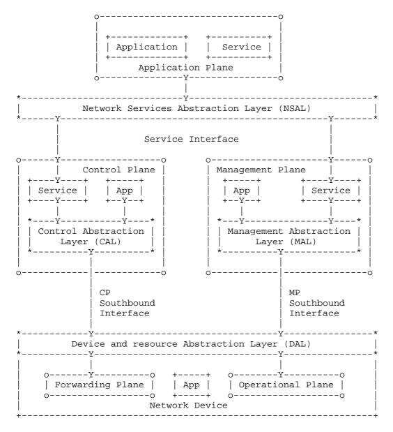
Figure 1: SDN Layer Architecture
