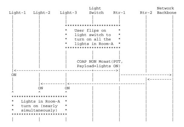
Figure 3: Light Switch Sends Multicast Control Message
