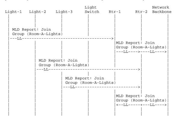
Figure 6: Joining Lighting Groups Using MLD
