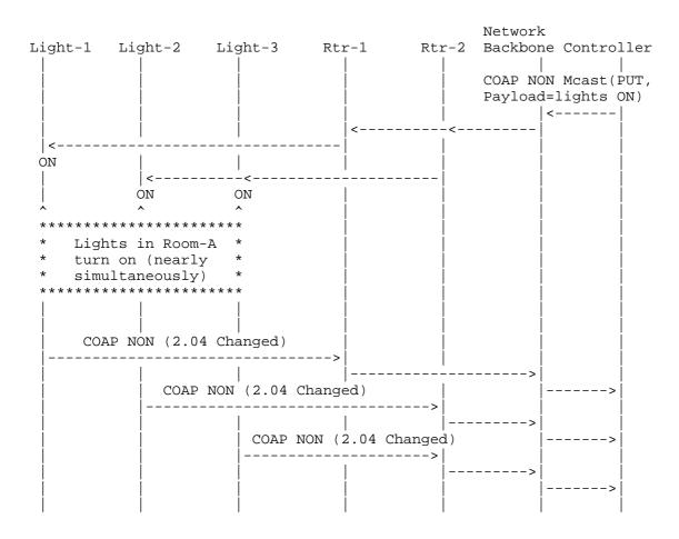
Figure 5: Controller on Backbone Sends Multicast Control Message
