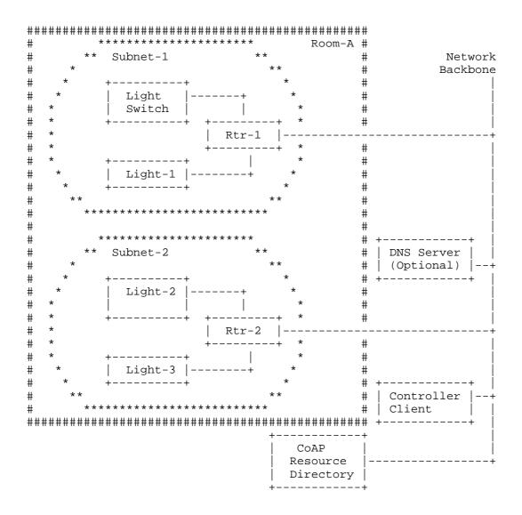
Figure 1: Network Topology of a Large Room (Room-A)
