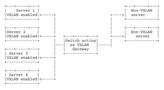
Figure 4: VXLAN Deployment - VXLAN Gateway
