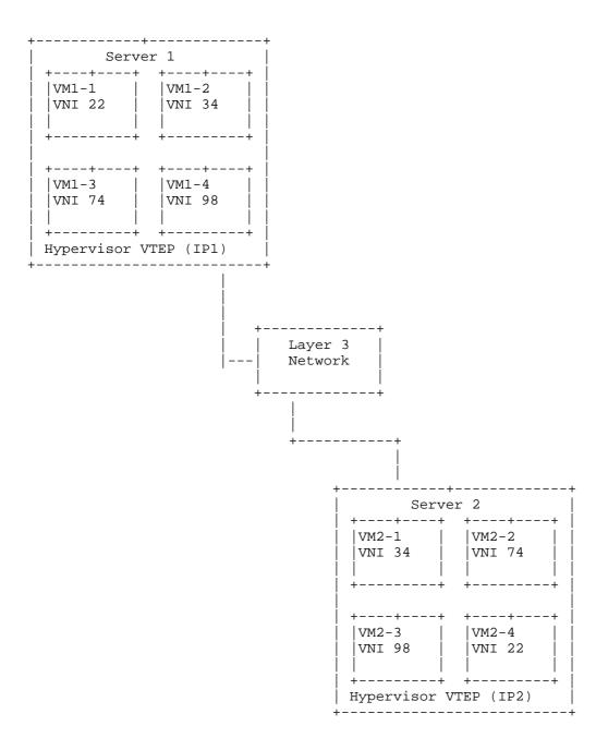
Figure 3: VXLAN Deployment - VTEPs across a Layer 3 Network
