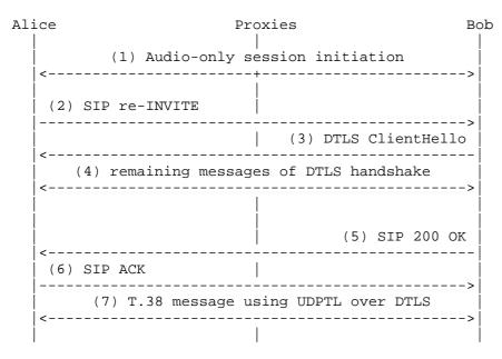
Figure 8: Message Flow of T.38 Fax Replacing Audio Media Stream in an Existing Audio-Only Session
