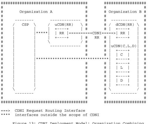
Figure 13: CDNI Deployment Model: Organization Combining CSP and Partial CDN
