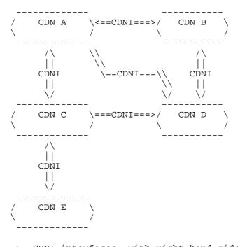
===> CDNI interfaces, with right-hand side CDN acting as dCDN to left-hand side CDN <==> CDNI interfaces, with right-hand side CDN acting as dCDN to left-hand side CDN and with left-hand side CDN acting as dCDN to right-hand side CDN
