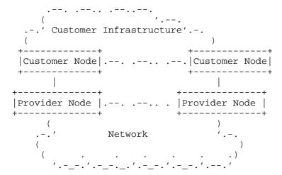
Figure 3: Reference Architecture: Connectivity Service Provided by the Same Network Provider Using Distinct Interconnection Nodes
