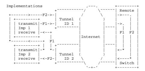
Illustrations of a test setup with a bidirectional tunnel. The upper diagram emphasizes the VLAN connectivity and geographical location (where "Imp #" is the sender and receiver of implementation 1 or 2 -- either Perfas+ or NetProbe in this test). The lower diagram shows example flows traveling between two measurement implementations. For simplicity, only two flows are shown, and the netem emulator is omitted (it would appear before or after the Internet, depending on the flow).
