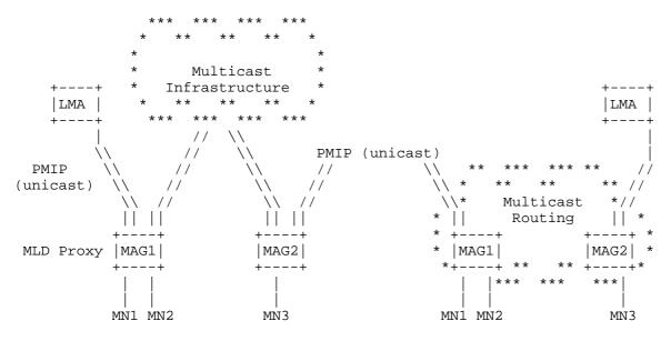
(a) Multicast Access at Proxy Uplink (b) Multicast Routing at MAG
